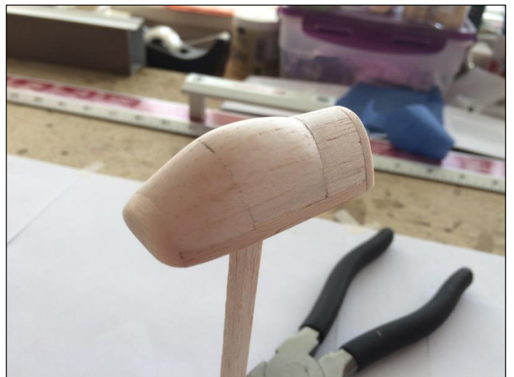
A new Photo Recce canopy with a rounded windscreen will be plunge-moulded, this is the canopy buck.
